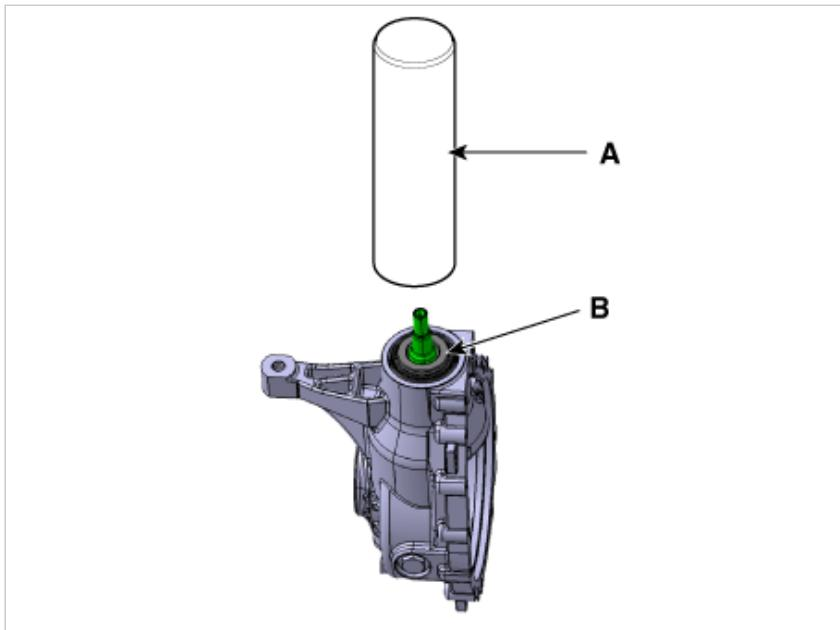
7. Using the SST (09530-3T600), install the pinion oil seal (A).
