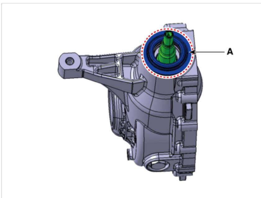
8. Using the round pipe and press, install the companion flange (A).
