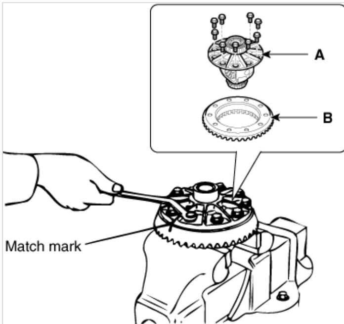
2. Using the SST (09474-4E200), remove the gear carrier bearing (A).
