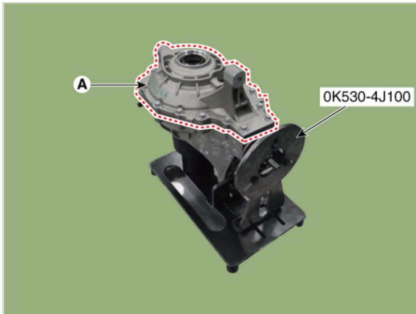
5. Remove the differential case assembly (A).
