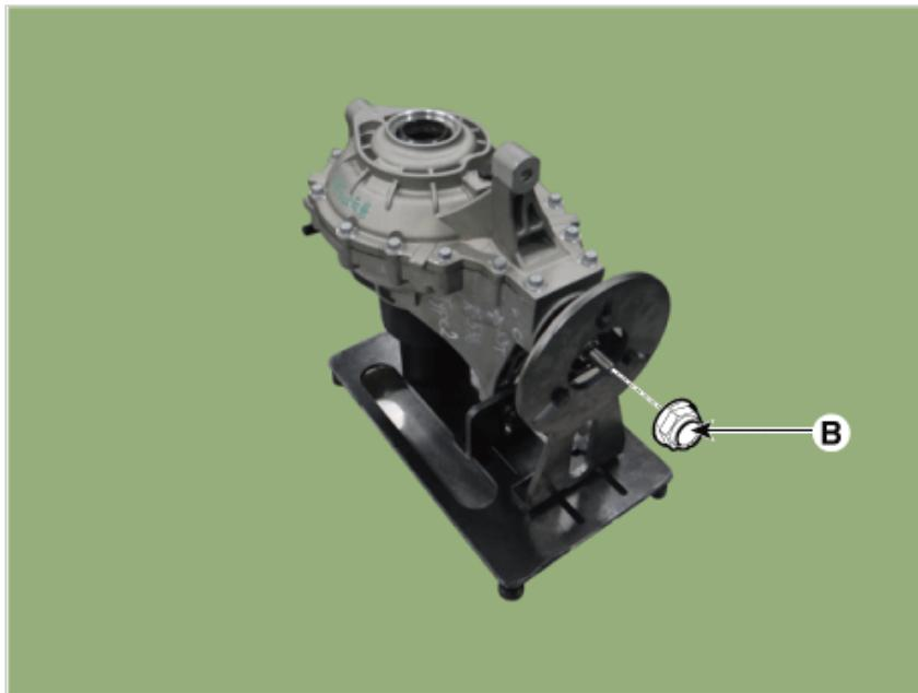
10. Install the pinion lock nut.
