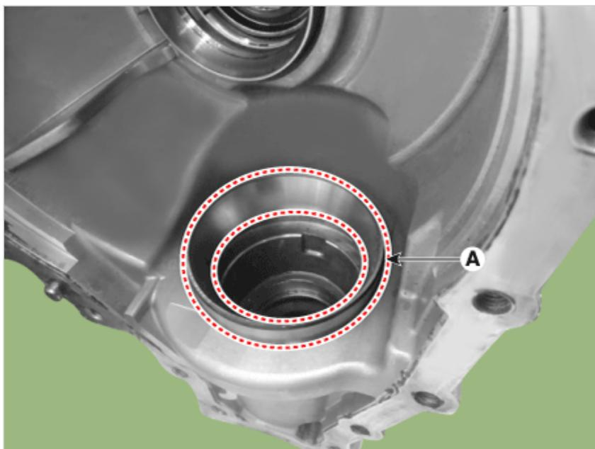
5. Using the press, remove the pinion rear bearing (A), the pinion gear adjustment shim (B) and the inner bearing adjustment shim (C) from the pinion drive gear in order.
