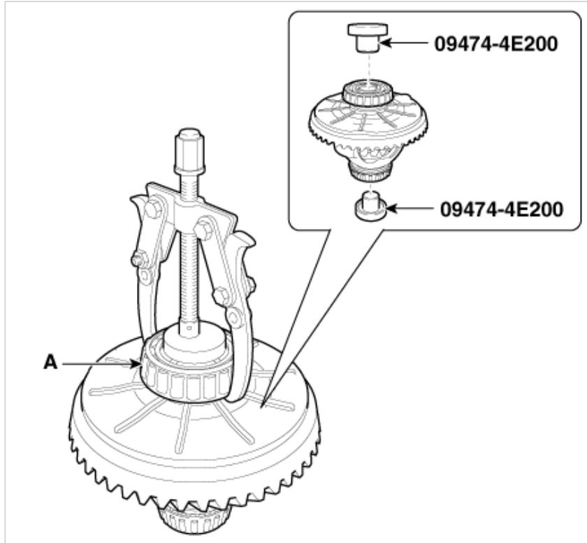
3. Remove the bearings and then attach "Left" or "Right" tags to each bearing.
