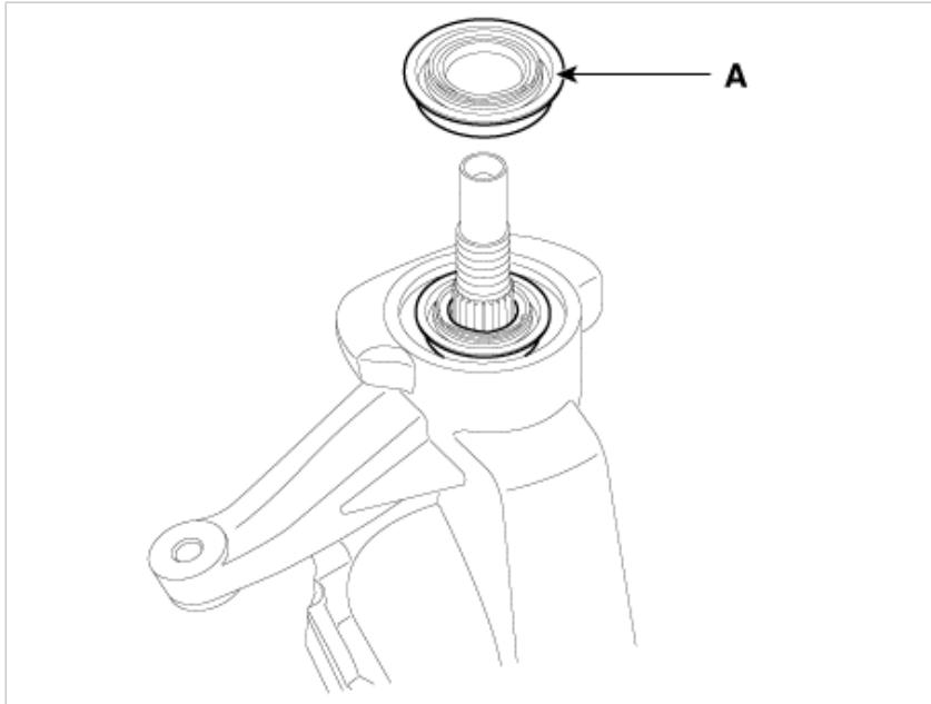
3. Using the press, remove the pinion drive gear (A).
