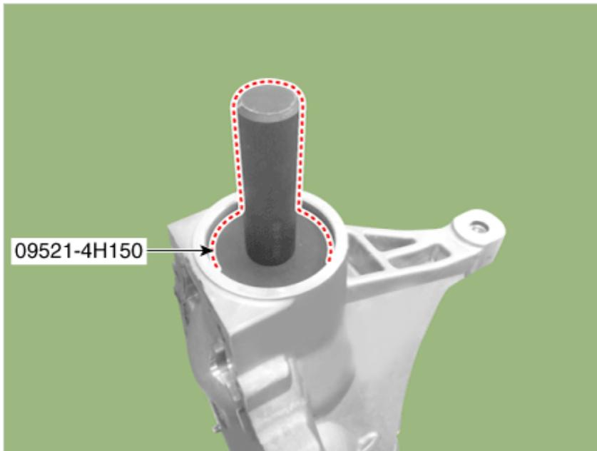
2. Using the SST (0K530-4J200), install the rear pinion bearing outer race (A).
