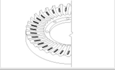
A diagram showing a cross-section of a ring gear with a uniform pattern of black marks across its width, indicating standard contact. |          |  |
