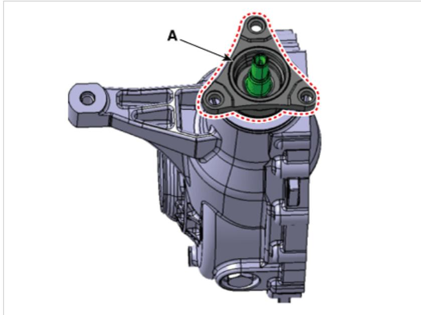
9. Using the SST (0K530-4J100), fix the companion flange (A) and then install the nut (B).
