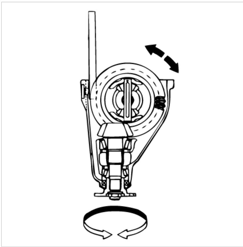
(3) Check the ring gear tooth contact pattern.
