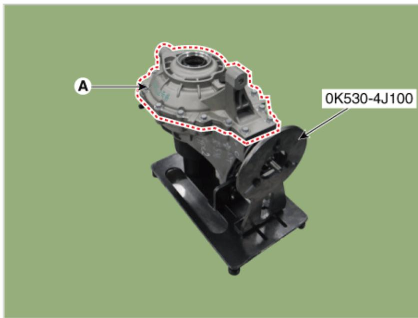
13. Using the SST (09530-3T500), install the LH,RH side oil seal.
