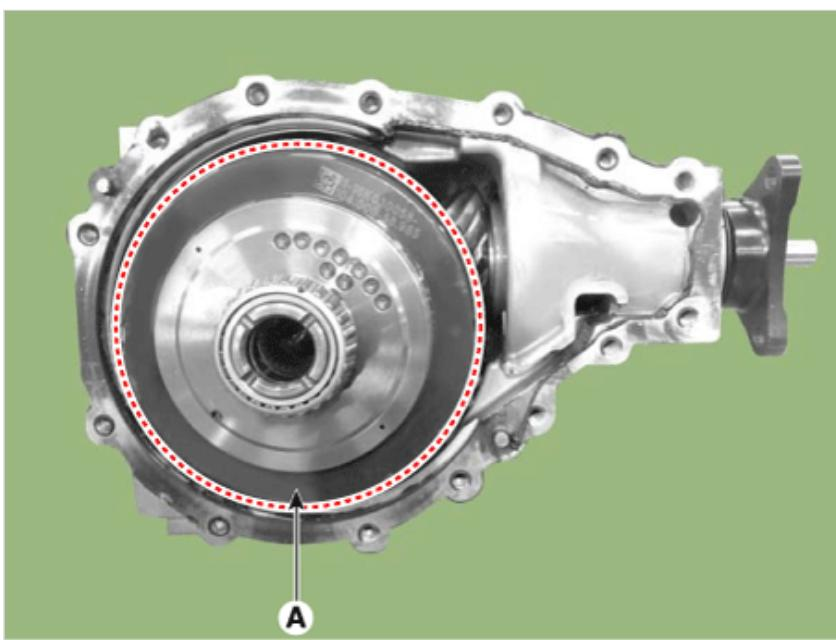
7. Using the SST (0K530-4J100), install the differential side cover (A).
