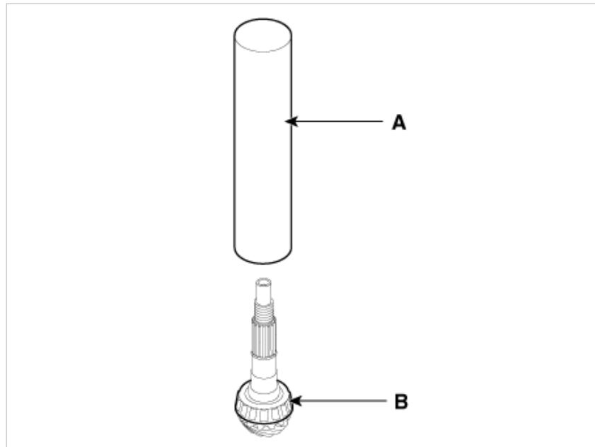
5. Install the Inner bearing adjustment shim (A) to the pinion drive gear (B).
