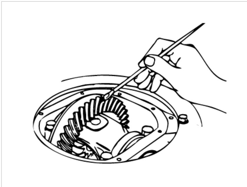
(2) Put the ring gear into the pinion drive gear while making each painted marks aligned, and repeatedly turn the ring gear or flange clockwise and counterclockwise to check if the gear teeth are engaged properly.
